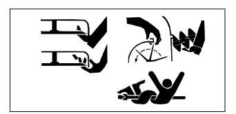
Keep hands and feet away while machine is running. Shut off power to service, lubricate or remove mower blades, augers or PTO shafts.
