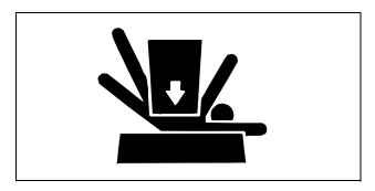
If you must work on a lifted machine or attachment, securely support the machine or attachment.
