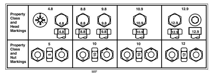
Class 4.8 Class 8.8 or 9.8 Class 10.9 Class 12.9 Lubricated Lubricated a Lubricated a Lubricated Dry a Dry a Dry a Dry a SIZE N•m lb-ft M6 4.8 3.5 4.5 6.5 8.5 9.5 11.5 14.5 **M8** 8.5 M<sub>10</sub> M12 M14 M16 M18 M<sub>2</sub>0 M22 M24 M27 M30 M33 M36
